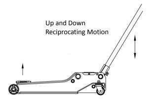
**CAUTION:** NEVER WIRE, CLAMP OR OTHERWISE DISABLE THE LIFT CONTROL VALVE TO FUCTION BY ANY MEANS OTHER THAN BY USING THE OPERATOR'S HAND. USE THE HANDLE PROVIDED WITH THIS PRODUCT OR AN AUTHORIZED REPLACEMENT HANDLE TO ENSURE PROPER RELEASE VALVE OPERATION. DO NOT USE EXTENSIONS ON THE OPERATING HANDLE.
