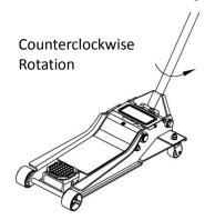
5. After removing jack from under the load, keep jack in the lowered position to reduce exposure to rust and contamination.
